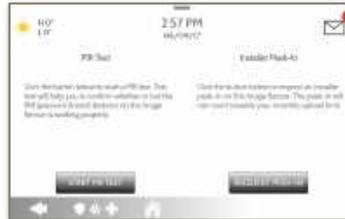
**PIR Test** checks the motion sensor
